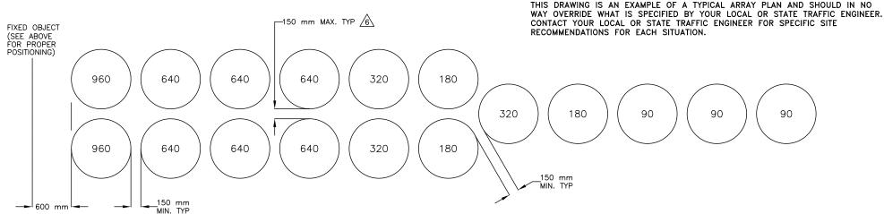
6 FOR FIXED OBJECT WIDTHS GREATER THAN 457 mm INCREASE SPACING OF DOUBLE WIDE BARRELS UP TO 305 mm APART.
