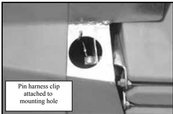
Pin harness clip attached to mounting hole
