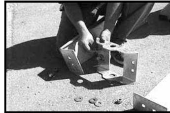
1.5 Attach the Adapter Straps to the Tie Strap Mount with the (4) 5/8" x 1 1/4" NC GRJ CADIPLTD bolts, and (4) Nylock Nuts. **The (4) washers are spacers and must be installed between the strap and the Tie Strap Mount as shown.**
